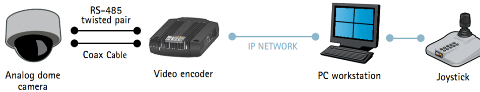
Figure (5): An analog PTZ dome camera can be controlled via the video encoder’s serial port (e.g., RS-485), making it possible to remotely control it over an IP network.
